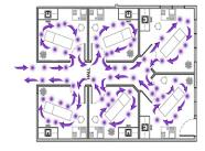
Current devices are placed in one, two or three positions using manual labor. The ADV Robot defeats the inverse square law since the Sterilray ADV moves autonomously to infinite positions within 18" of all surface with no "blind" spots. Closer means superior disinfection: 10 to 1000 times better than current methods in less than 1/2 the time.
